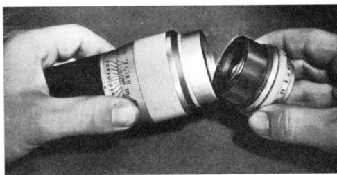
Figure 32. Removing the Hektor 135mm. lens assembly from the mount.
