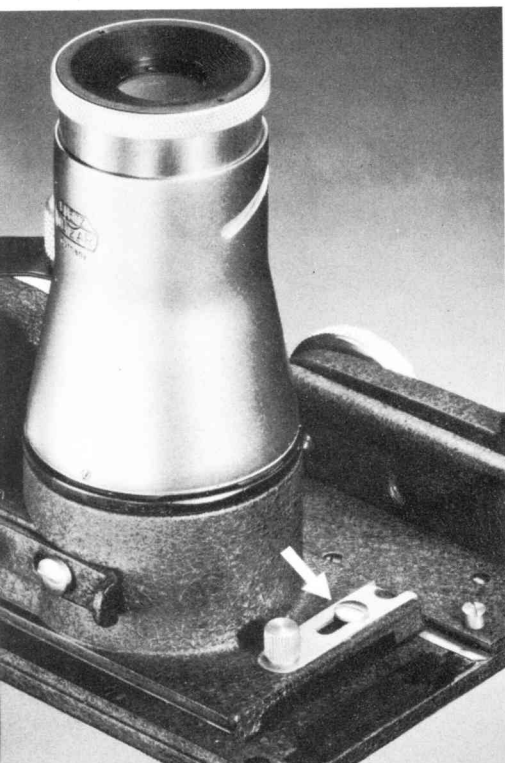
Figure 11. Locking lever at full forward position for removing sliding plate.
