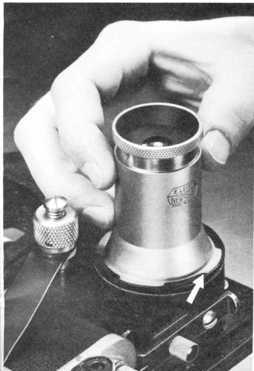
Figure 9. The four bayonet flanges of the 5x Magnifier fit the bayonet catches.
