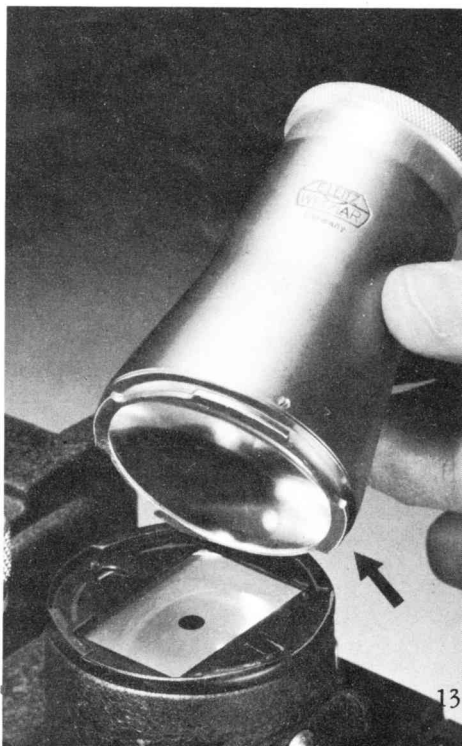
Figure 10. The large wide field magnifier is similarly fitted to the bayonet catches.
