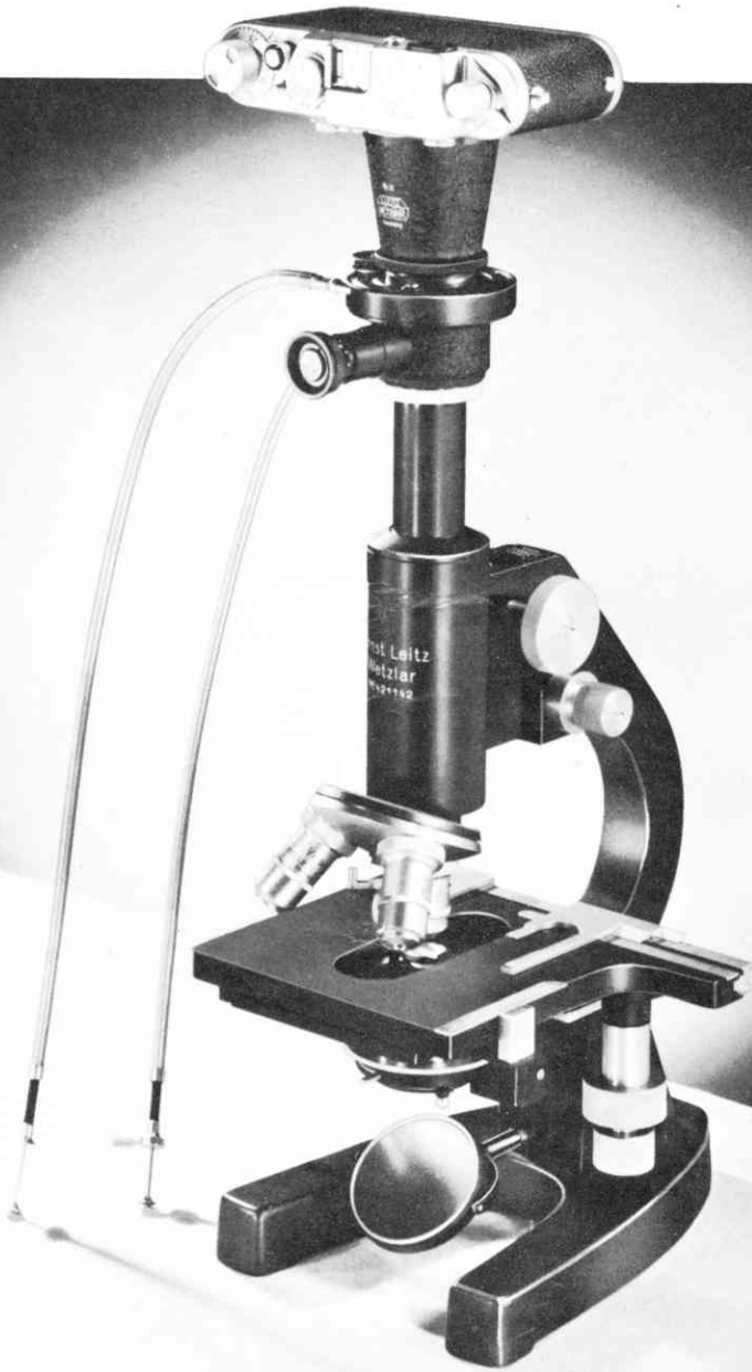
Figure 29. The Leitz GO 48/77 microscope fitted with the Micro-Ibso attachment and the Leica camera model IIIf.
